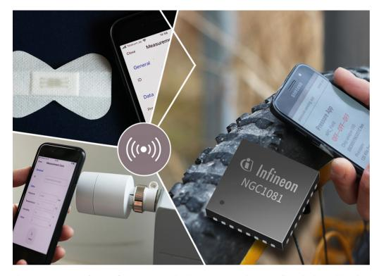
The new NGC1081 from Infineon is a single-chip NFC tag-side controller which enables the IoT industry to develop low-cost, miniature edge computing and sensing devices.
